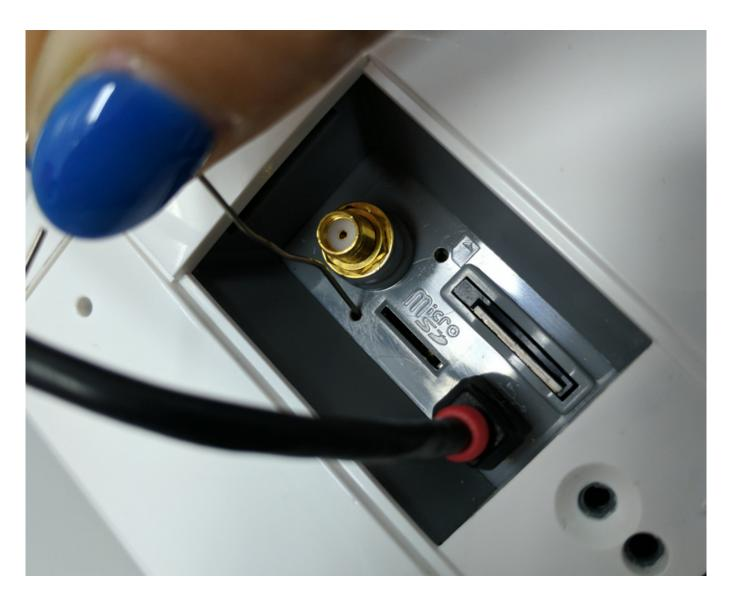
1.5 Remove the paperclip, and a new hard drive will appear on your computer labelled MEZZO-BOOT:
